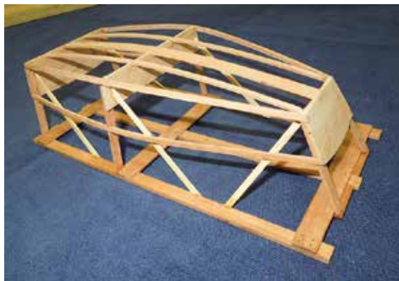
Tim's Optimist Pram as the originals were built, on a jig.
