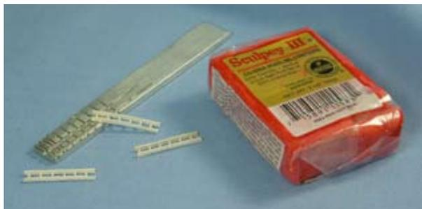
**Ladders made by pressing Sculpy into a purpose-made aluminum mold.**
