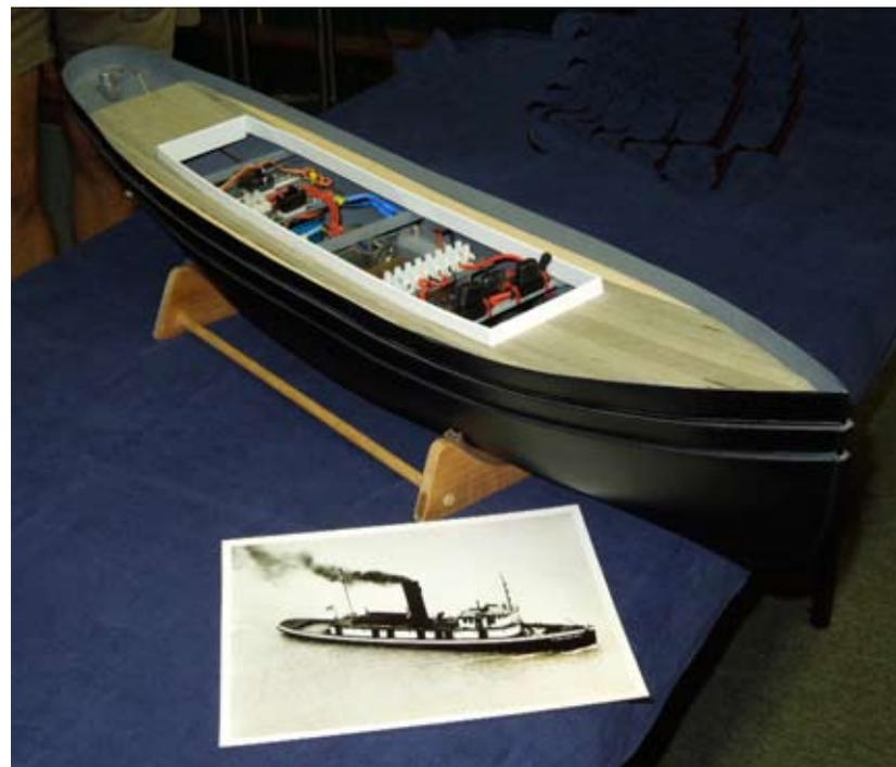
Howard Howe's, rendition of the 1919 tug, *Buttercup*. \*Howard says he has her set up with one electronic speed controller to supply the voltage to both motors. So, except for minor variations in construction of the two motors they should basically run at the same speed with the same voltage applied, so neither should be a drag on its mate.
