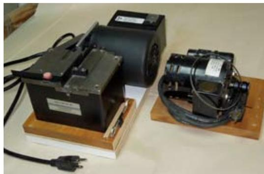
Repowered PREAC saw; 1/8 to 1/3hp.
