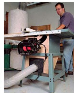
Table saw dust and chip collectors
