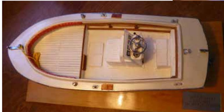
The "better way" to apply graphics to this hull is by laser-printing the graphic in reverse and using Mod Podge product to adhere. When dry, the paper is wetted, then rubbed off, leaving the ink on the surface.
