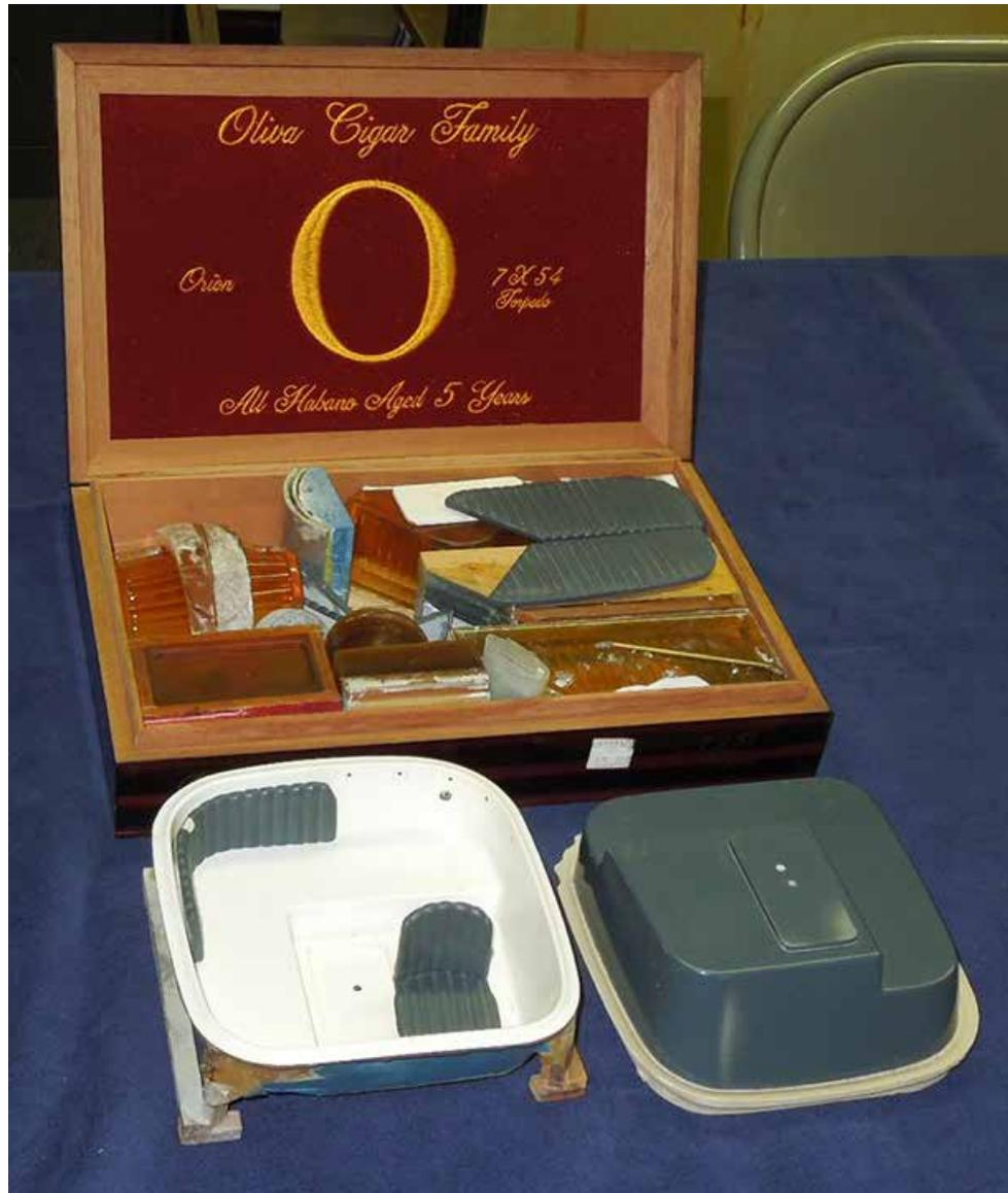
**Curtis Miller** displayed more of his highly professional fabrication of *DONZI* models. Curtis explained how he created these hulls and power train components, with patterns, molds and castings. Specifically, the outdrive pattern is wood.
