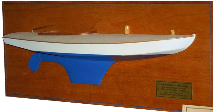
*Fish Class Yacht* rendered in Dow Styrofoam on a basswood center plate, with nameplate cheaply rendered by a laser printer.
