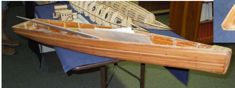
Chuck LaFave planked this Marblehead 50/800 RC hull with Home Depot Cedar.
