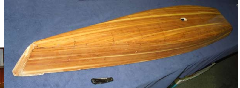
Chuck LaFave planked this Marblehead 50/800 RC hull with Home Depot Cedar.
