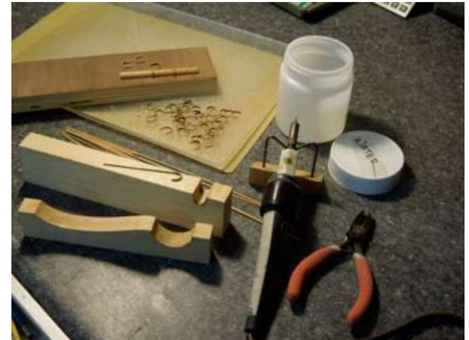
This is the set-up for making half mast hoops of bamboo that was taped but ended on the cutting room floor. The producer was more interested in feelings and finished product than the building process involved.
