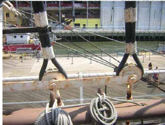
**Sheer poles in a variety of materials and shapes prevent deadeyes and their equivalents from rotating due to shrouds in tension. Photos by Phil.**
