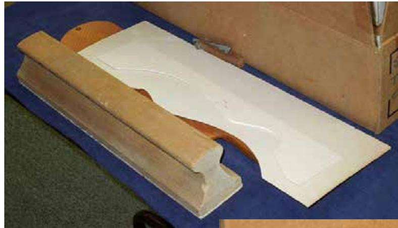
Curtis showed a variety of tools he has used for layout, lofting and dressing 1:1 hulls and suggested that the methods can be scaled for models.
