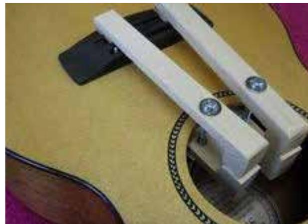
Here's a good principle for making deep planking clamps. An improvement would be to slot the ends vertically and insert a bit of flat stock to keep the clamp arms aligned.
