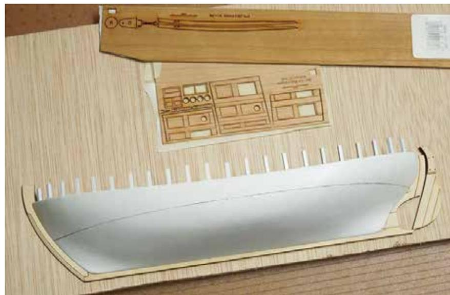
Sec/Ed's Gerda III in process. Top two show the HDPU hull roughed out with bandsaw. Bottom two with timberheads in place and some of the laser parts, then with the timberheads filled and hull primed.
