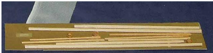
Left are blanks for turning the masts, held together with School glue stick and split apart to form halves, after being turned in a pistol drill.
