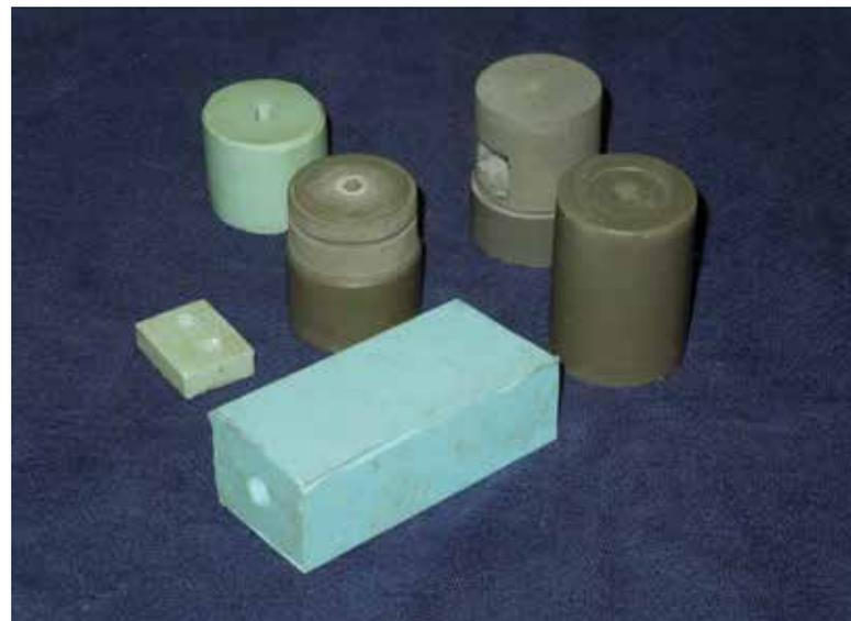
Skipper Ed discussed and showed samples of his casting materials and techniques, using metal filled resins and RTV.
