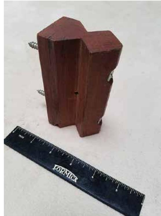
Brad's half-hull grabber allows positioning of the baulk, in your vise, in a variety of orientations.
