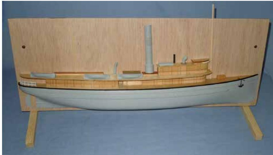
This is a temporary stack-up of SS *Mascotte* parts. The hull is BONDOLITE, cast into a Plaster-of-Paris mold. Anchor below is an assembly of laser-cut, 1/32" acrylic parts.
