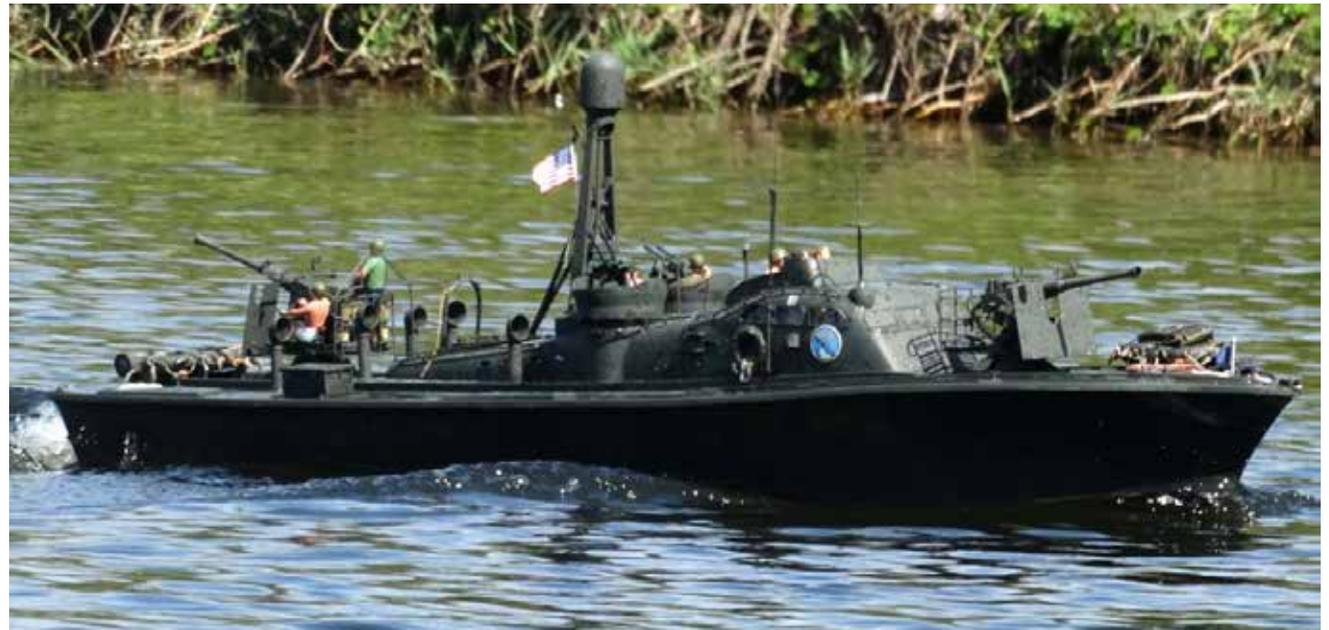
**PTGB-61, researched and modeled by Lew Zerfas. One of three conversions from patrol-torpedoe to full gunboats. "Used" 77 foot Elcos were modified on station to be used against shallow-draft smaller craft and barges against which torpedoes and depth charges were innappropriate.**
